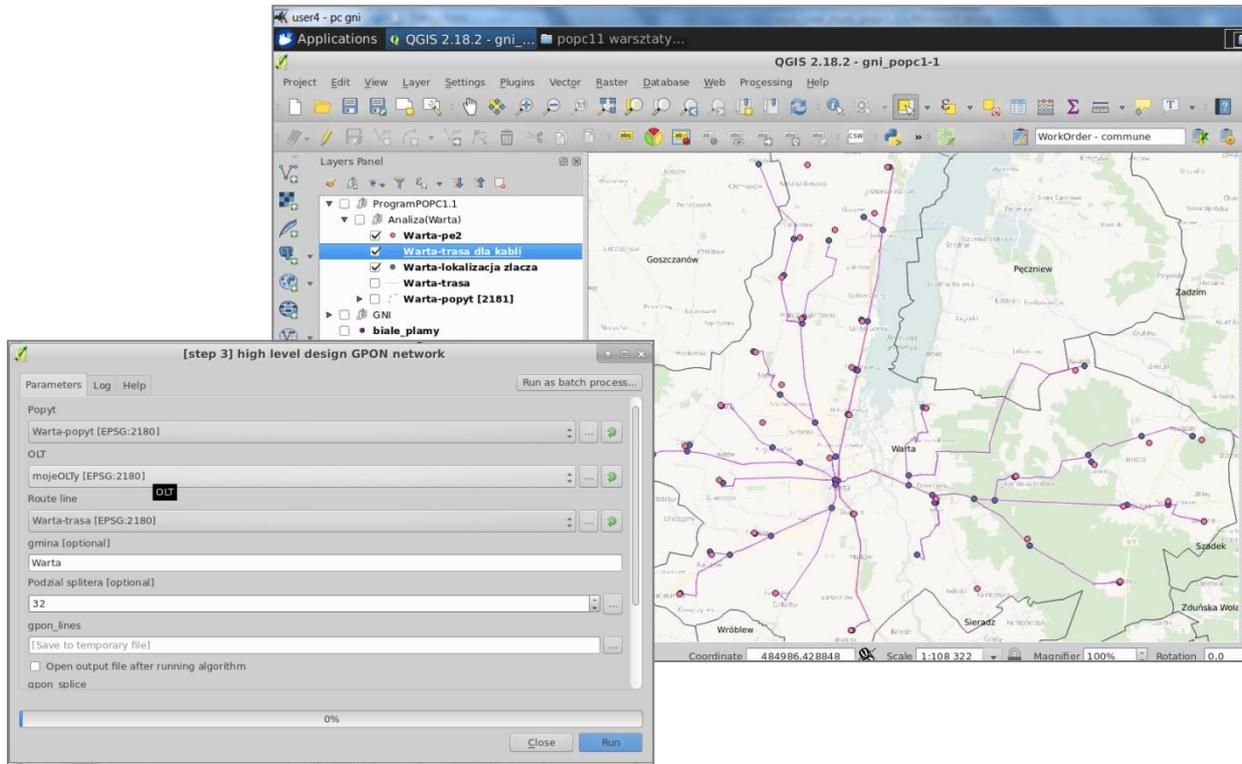
Using the cable routing layer and Dijkstra algorithm, *wizard* develops a route proposal concerning optical fiber cables and optical fiber connectors. The data is enriched with information that enables the construction of a network plan. The user can adjust the location of the splice closures and determine the hierarchy of the developed network.
