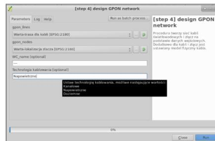
Upon the completion of the algorithm, in QGIS there are geometry objects representing planned cables and splice closure locations. Additional information such as the length of the cable and its fiber profile is added to stored data. This information is calculated from address points being used. The algorithm also supports versioning of concepts developed within the chosen work context.
