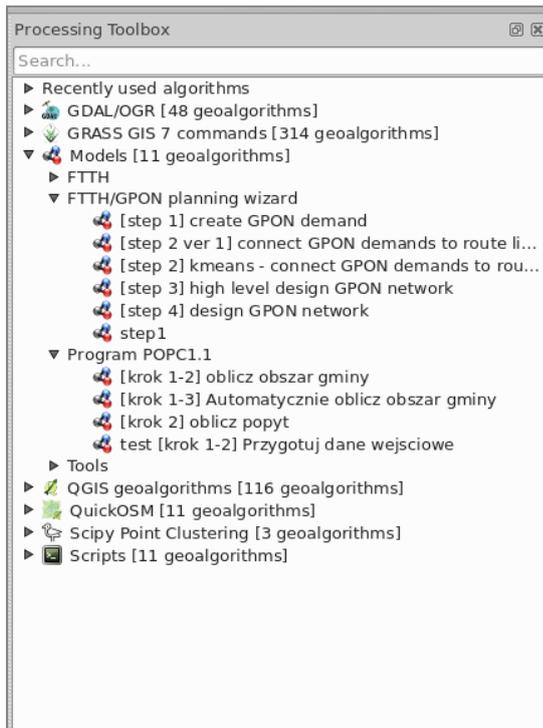
The entire solution was based on the concept of so called wizards which realize the process of preparing the FTTH network technical concept step by step. Using 'geoprocessing' modeller, we created models requiring only the necessary input data and parameters to be provided at the beginning. Algorithmic complexity was encapsulated within models in the form of designed flow, which use existing algorithms and calls dedicated scripts.
