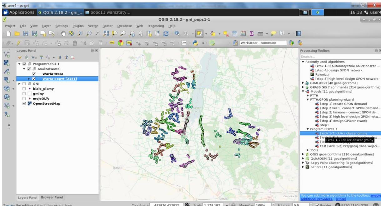
During the following stages of working with the tool, the user initiates the step of high level network planning. At the beginning the user provides layers prepared in the previous steps and a layer with starting point (OLT), from which the GPON network will be fed.
